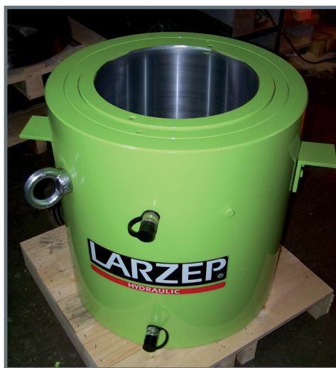
DDR200015 cylinder. 2.000 Tn capacity cylinder to place a load cell for pile testing.
